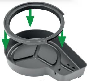
3. Fit the four GoGro Valve Pillar Supports into the base of the tray.
