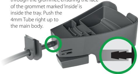
**Top tip:** we advise you do not cut down the 4mm Tube required for connecting the tray to the first line until you have confirmed your system configuration.
