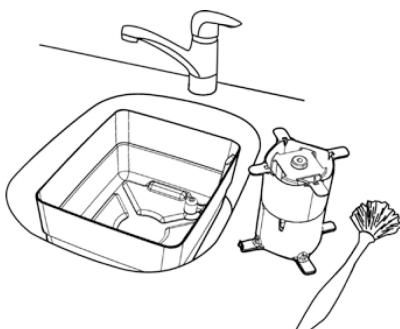
3. Wash the cover, water lid, tank and sprout lids warm water with a mild disinfectant to kill any unwanted bacteria. Clean the pump gently with a cloth or brush. When storing your *Aqua Garden by PLANT!T* for an extended period of time it is advisable to clean it thoroughly! Embedded dirt and sediment from the nutrition water will be difficult to remove later when dry!
