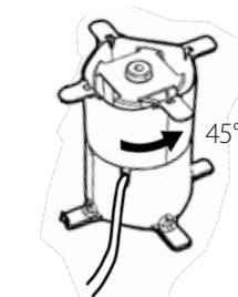
7. Position the top and base part of the support column on top of one another, then turn them 45° anticlockwise. Push the pump gently from the top with a finger to attach the suction cups on the pump to the base of the support column.
